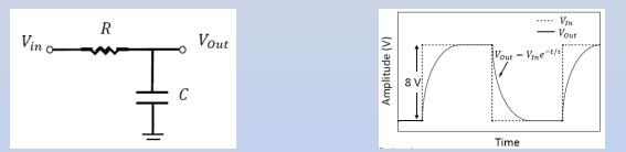
• Frequency response of RC circuits to AC signals.
